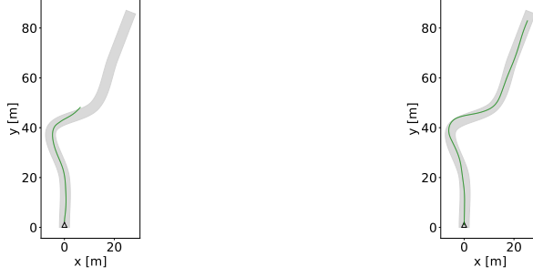
Fig. 7: Example of a disagreement scenario. Left: Vehicle simulated in BeamNG leaves short segment heading towards following segment. Right: Vehicle simulated in Donkey stays within the lane.
