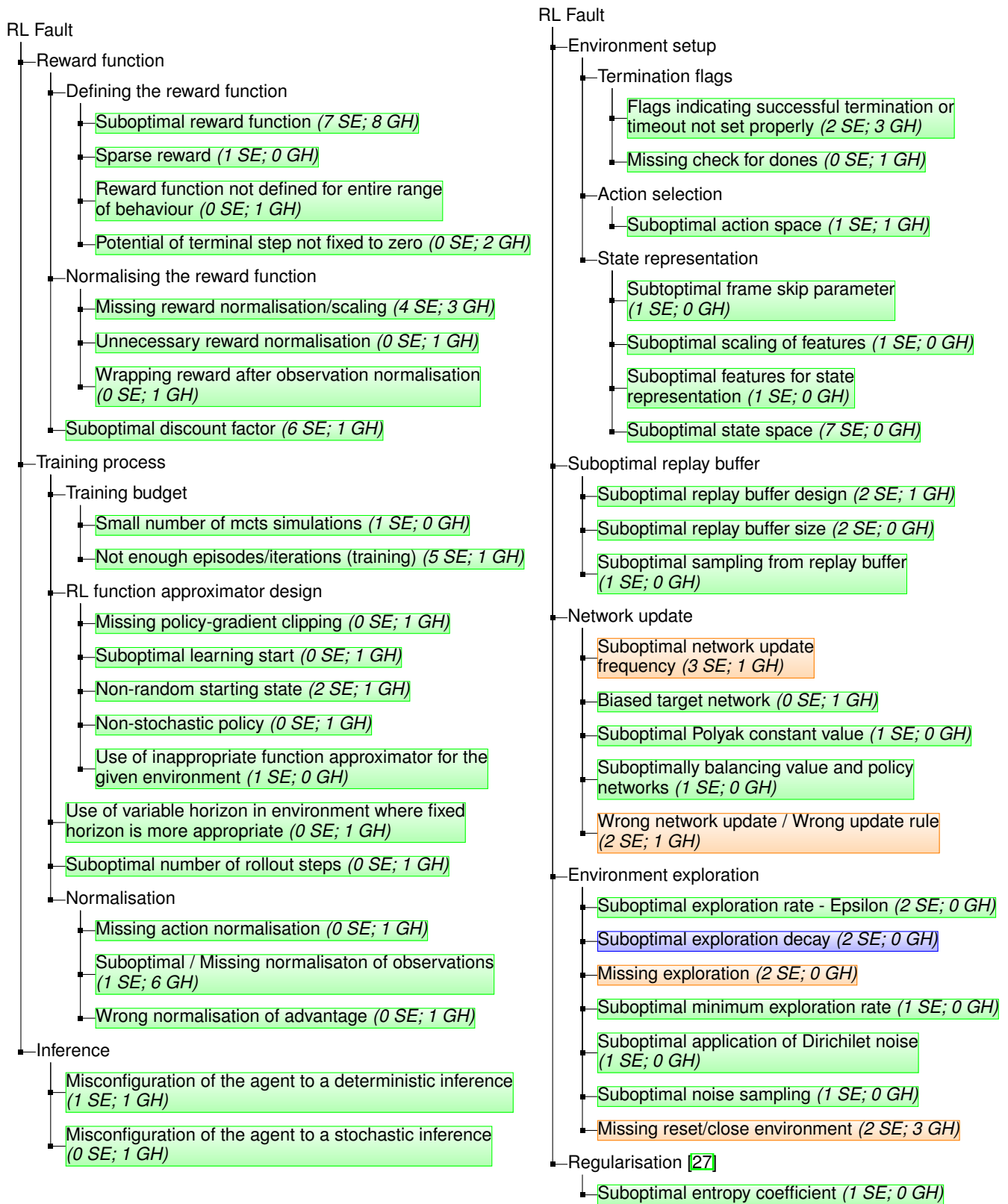
Fig. 1: Taxonomy of real RL faults: green indicates new fault types; orange and blue indicate fault types in common with the previous taxonomy [8]; blue indicates the ones that we renamed. SE/GH are preceded by the number of instances found in StackExchange/Github.
